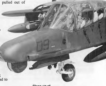
Close-up of the extended nose and AN/AAS-37 FLIR/LASER turret on the upgraded OV-10D. The OV-10D also has uprated engines and ordnance-mounting features and capabilities that enhance its military capability. **Photo: Norman Taylor**
